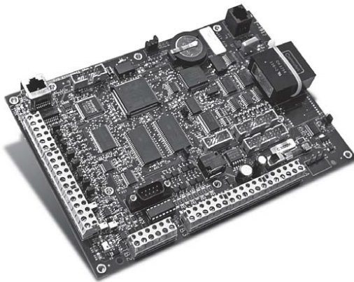
Orenco® TeleComm™ (TCOM) ATRTU-NET remote telemetry board
